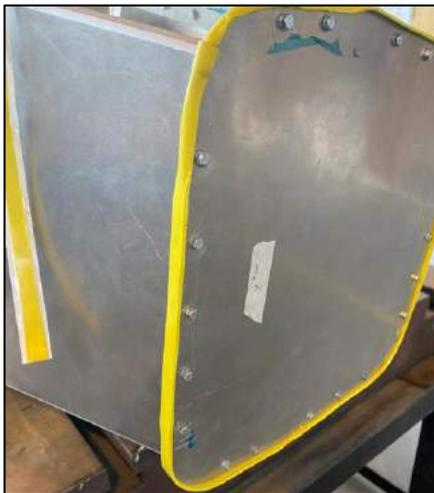
Figure 40 Gum tape around sharp outer edges.
