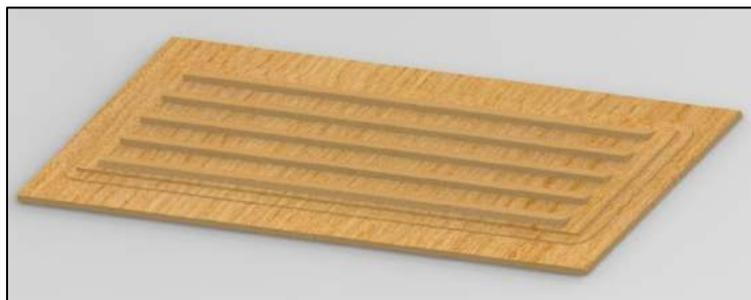
Figure 52 Louvre MDF mould.
