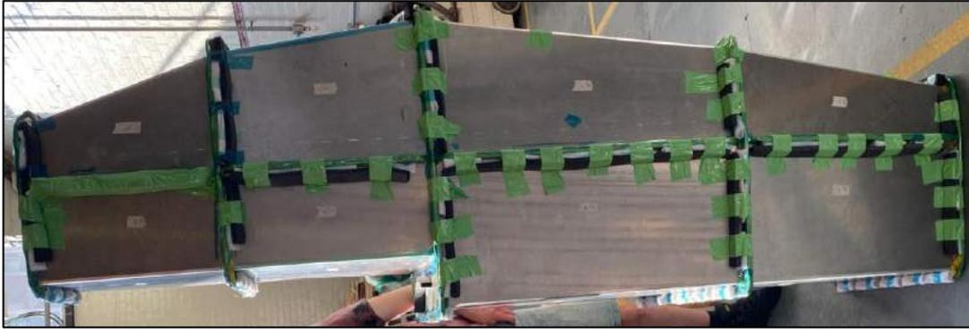
Figure 42 Rubber and flash tape to cover bolts.
