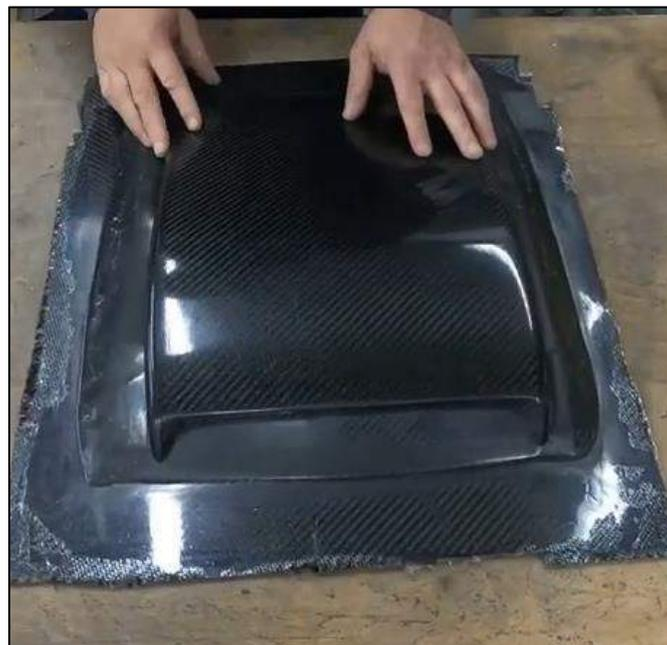
Figure 55 Hooded vent to be post processed to correct size.
