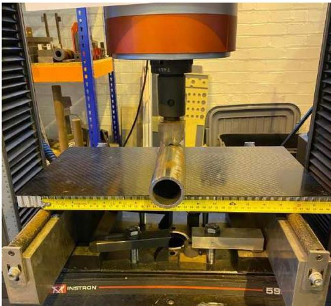
Figure 30 Instron three point bend test.
