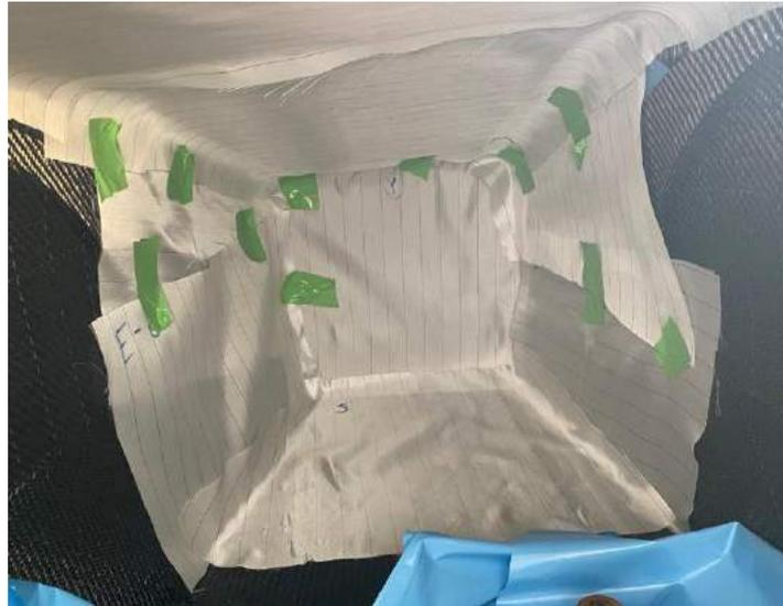
Figure 46 Peel ply secured with flash tape.
