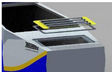
Figure 15 Louvre on the engine bay cover.
