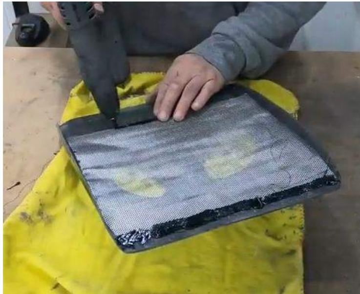
**Figure 56 Mesh superglued onto cured carbon fibre,**
